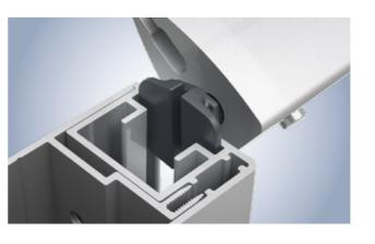
Safely guided – even in winds In winds the elegant bottom rail profile at the bottom of the awning revolves too so that the system runs **reliably and quietly** without jamming. This protects the fabric and mechanism and extends the operating life of the whole system.
