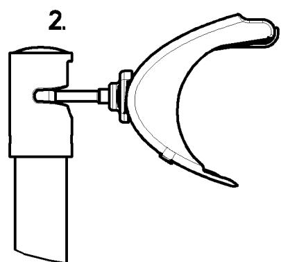
Loosen the hand knob on the wind support (3.), and slide the rotating head upwards (approx. 20mm) until the awning is slightly tensioned against the drop profile (4.). **Do not turn the rotating head during this time.** Then re-tighten the hand knob (5.).
