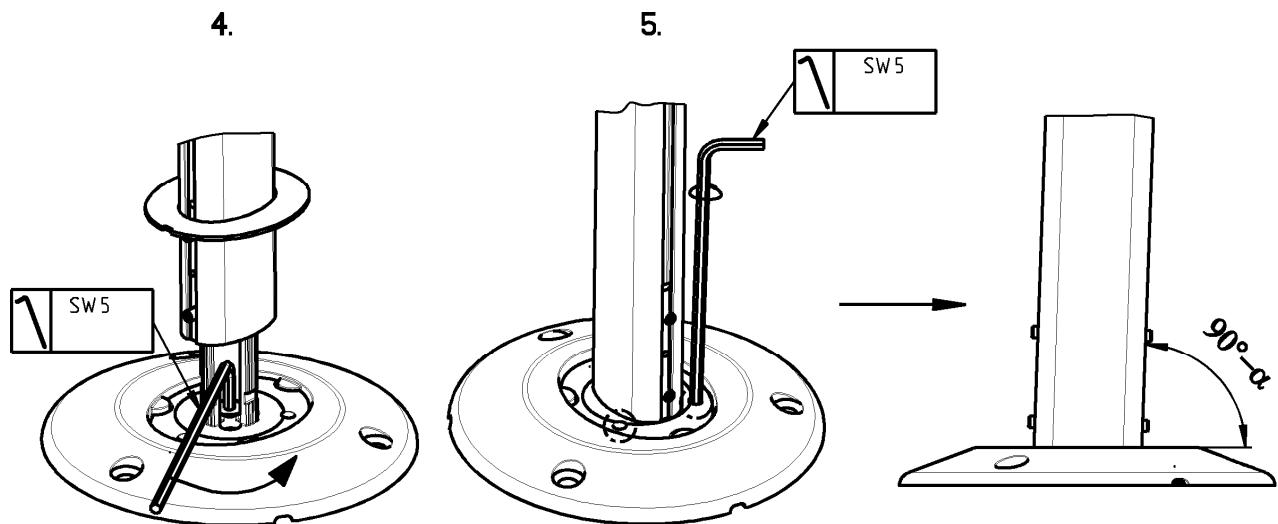
Once the required angle is reached, re-tighten the screw located in the centre of the adjustment base (4.) and re-tighten the four grub screws at the bottom end of the wind support (1.)
