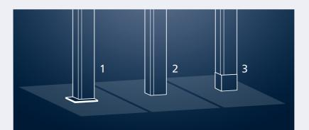
1: Visible post plate with a cover 2: Concreting or post plate in the ground 3: Height-adjustable post
